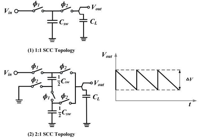
Fig. 1. SCC topology with different conversion ratios.
