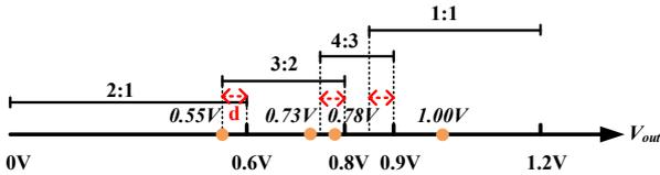
Fig. 4. The output voltage range is divided into several regions, where each region stands for different possible ratio could be employed. And the yellow points on the axis represent four different load voltages.
