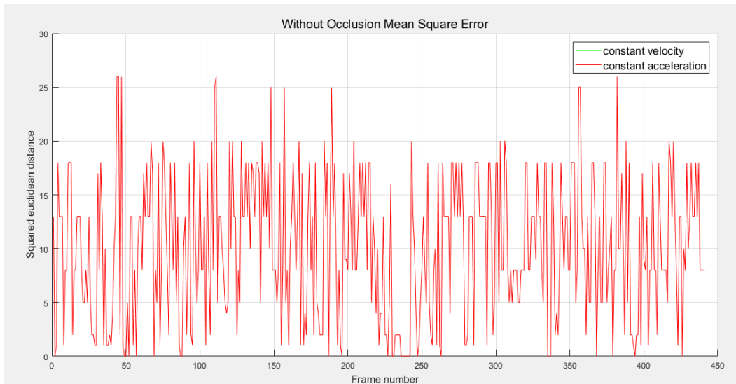
Figure 4. Without Occlusion Mean Square Error
