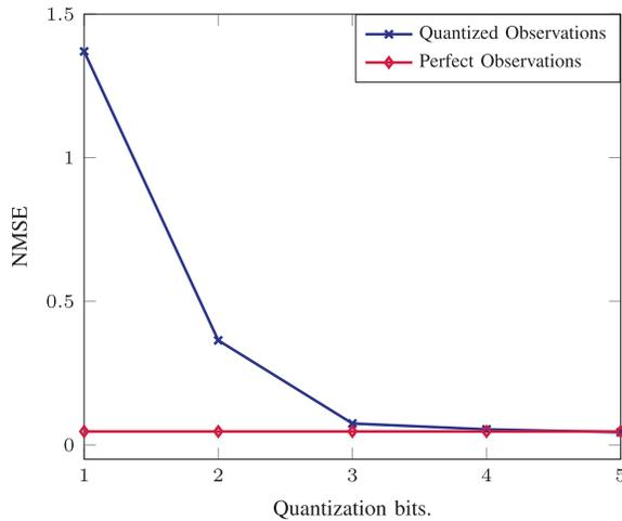
Fig. 8. The estimation error versus number of quantization bits.
