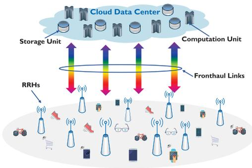
Fig. 1. The architecture of Cloud-RAN with massive mobile devices, in which, all the RRHs are connected to a single BBU pool through high-capacity and low-latency optical fronthaul links.
