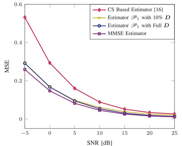
Fig. 3. Mean-squared error versus transmit SNR with  $T = 30$ .
