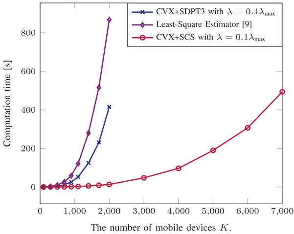
Fig. 7. Computation time versus the number of mobile devices.
