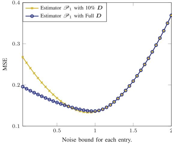
Fig. 4. Mean-squared error versus noise bound for each entry (the underlying noise variance is 1 for each entry).
