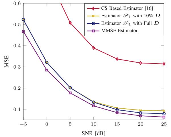
Fig. 2. Mean-squared error versus transmit SNR with  $T = 10$ .
