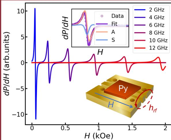
➤ The FMR curves are fitted using a derivative Lorentzian: (Antisymmetric + Symmetric + Offset)
