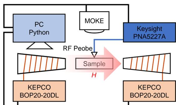
One-port S11 measured on a probe station with in-plane dc field applied along the easy axis. All measurements were carried out at room temperature.
