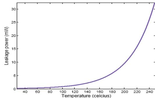
**Fig.2 Relation between leakage power and temperature**
