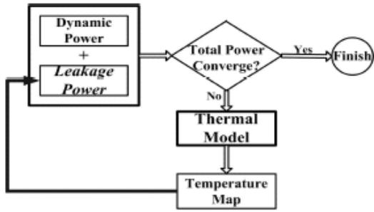
**Fig. 3 Full-chip thermal model closes the loop for accurate leakage power calculation**
