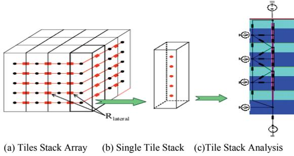
**Fig. 1 Resistive thermal model for a 3D IC**
