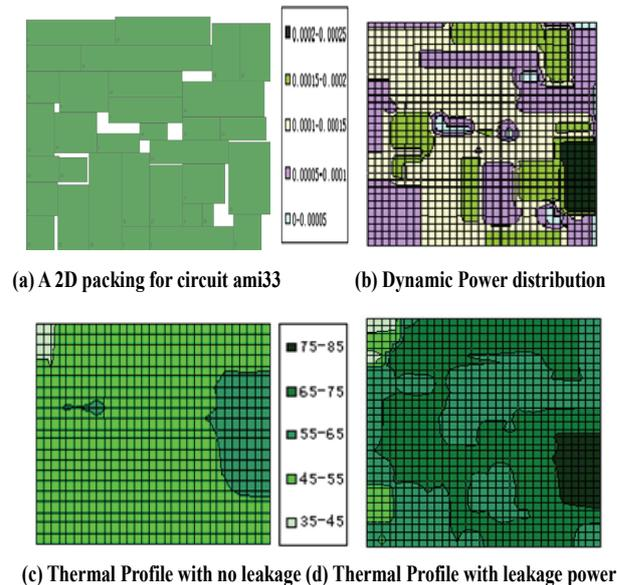
**(c) Thermal Profile with no leakage (d) Thermal Profile with leakage power**
