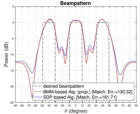
Figure 3. Transmit beampattern design with 3 targets .
