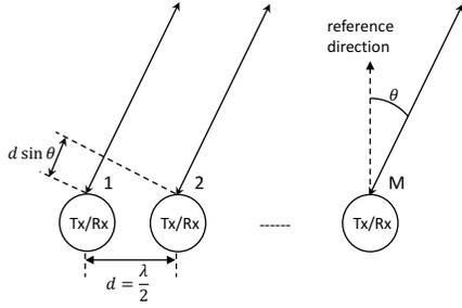
Figure 1. MIMO transceiver with  $M$  antennas ( $\theta$ : spacial direction of interest).
